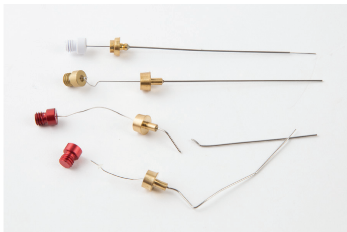
Figure 1: SPME fibers break easily during routine operation.
